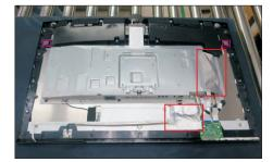
Use a Philips-head screwdriver to remove 2pcs screw for unlocking the USB board, and disconnect the two USB FFC cables from the connectors of the board, then release the USB board from the hooks of the middle frame. Tear off 1pcs aluminum foil for unfixing the touch FFC wire, and then disconnect LED wire from the connector of the board.
