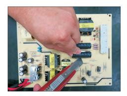
S23-2 Ensure cutting path within the glue, don't touch bulk cap. or PCB.
