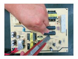
S23-4 Take out bulk cap. pin solder with soldering iron and absorber.
