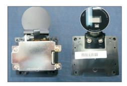
Use a Philips-head screwdriver to remove 18(13+5)pcs screws for unlocking the middle bezel with the panel, to remove 4pcs screws for unlocking the bracket with the panel, to remove 1pcs screws to unlock the heat-sink with board.
