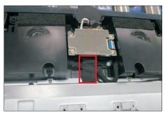
Tear off tapes of camera FFC cable, then disconnect the cable from the connectors and remove it. Tear off 2pcs acetate tape, then disconnect the Mic wire from the connector of the board.
