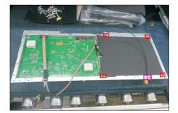
Use a Philips-head screwdriver to remove 8pcs screws for interface board and power board. Release the panel lamp cable from the hook of the bracket.
