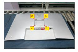
Tear off screen protector, then wedge your fingers between rear cover and the middle bezel on the corners of the top side of the monitor to release the rear cover, then use one hand to press the middle bezel, the other hand to pull up the rear cover in order of arrow preference for unlocking the rear cover.
