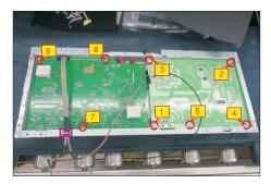
S22 Remove the power board and interface board from the bracket chassis module carefully, and then disconnect all of the cables.
