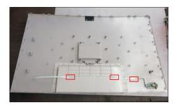
Tear off 2pcs sound-absorbing foams from the left and right speakers' screws, then tear off 2pcs aluminum foil to uncover all the connectors.
