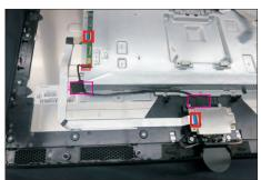
Use a Philips-head screwdriver to remove 8pcs screws for unlocking the camera unit with the middle frame, then remove it and put it aside.
